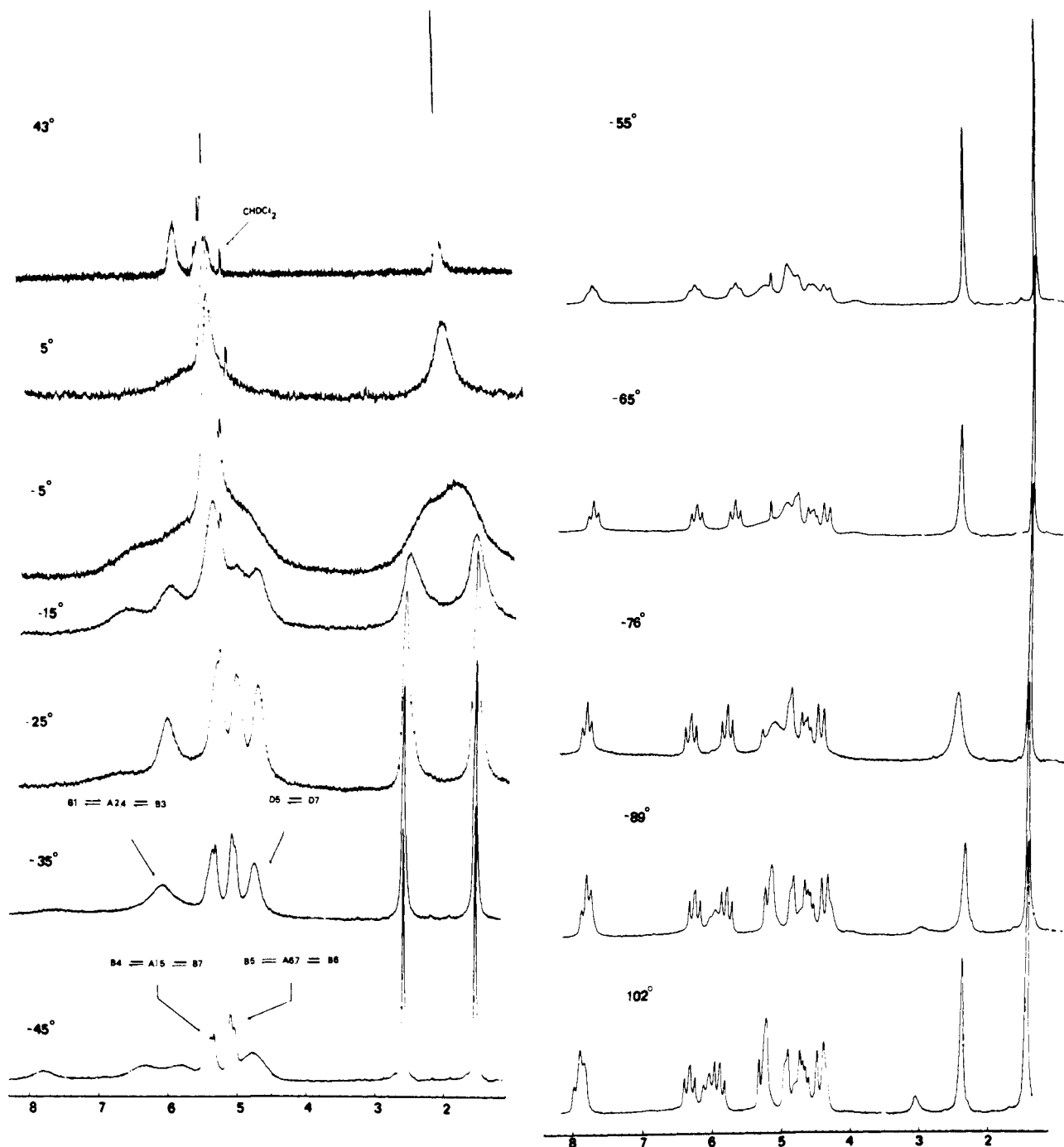
Figure 2. Variable-temperature ^1\text{H} NMR spectrum of methyltropyliumiron tricarbonyl from -102 to 43 ^\circ\text{C} . Solvent changes were necessary to span this temperature range and are indicated in the Experimental Section.
